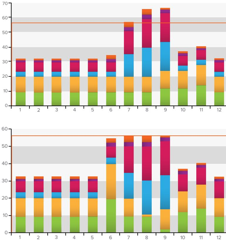
Figure 5. Ideal loading for packing line (top) and feasible loading on packing line considering available capacity (bottom). Each color represents load generated from a product or group of products.
